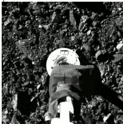
Robotic arm of OSIRIS-REx picks up a sample from the asteroid Bennu.
